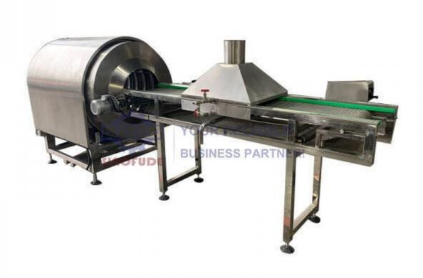
Sugar Coating Machine (Sugar Sanding Machine)
